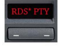
To activate RDS, press the left button under the RDS option. The radio program type will be displayed for a few seconds.
